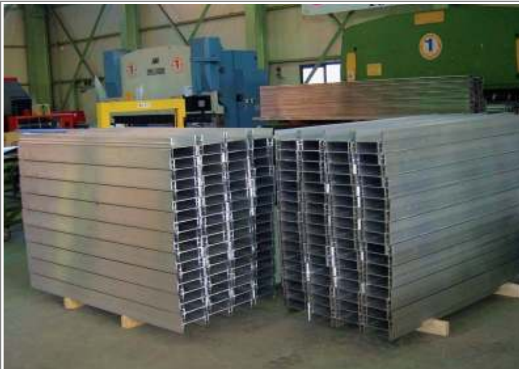
Large size strut and Raw Material Storage Area
